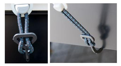
Use the elastics with hooks at the rear and attach them to the chassis or the support feet (depending on which model you have):
